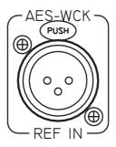
This XLR type connector has two functions. It can accept an AES/EBU sync reference or any Word-Clock signals. When the DUA II is set to AES synchronization mode, it will resolve the DUA II clock to the AES/EBU sync signal present here. When DUA II is set to Word-Clock synchronization mode, it will sync the DUA II clock to the Word-Clock signal present here.
